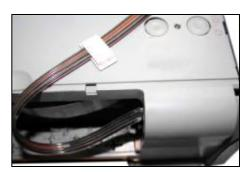
Place the tube through supporting arm. Move the cartridge car to left end and right end. Make sure that the tubes are not too tight or too loose.
